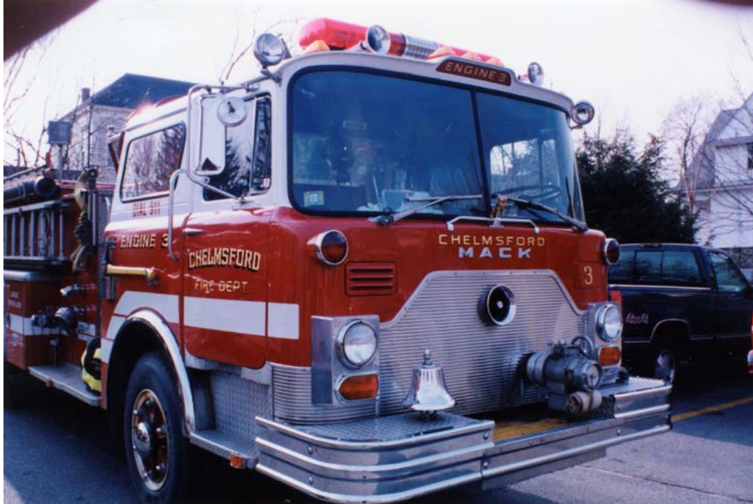
This is the 1981 Mack CF 1000 g.p.m. Pumper, Engine 3, as it looked circa 1996 with new graphics and light bar (Chelmsford Fire Department Collection)
