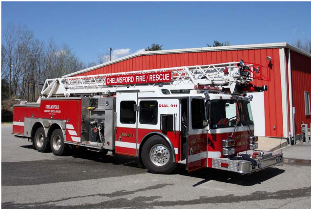
2001 Central States Quint Ladder Truck/Pumper on HME Chassis, Engine 1, behind East Chelmsford Fire Station. The siren-horns are built into the front bumper to protect the firefighters' hearing while on the road (2011 photo by Fred Merriam)
