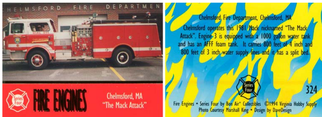
1994 Collectible Fire Engine card by the Virginia Hobby Supply Company The subject of this card is the 1981 Mack CF 1000 g.p.m. pumper, Engine 3, at West Chelmsford (Chelmsford Fire Department Collection)
