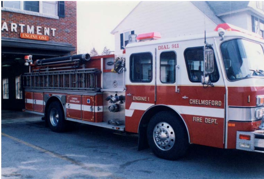
1989 Emergency-One/Hush 1250 g.p.m. Pumper with 750 gallon tank, Engine 1, had its engine behind the rear wheels and was known as the "Hush" due to its quite ride (Chelmsford Fire Department Collection)
