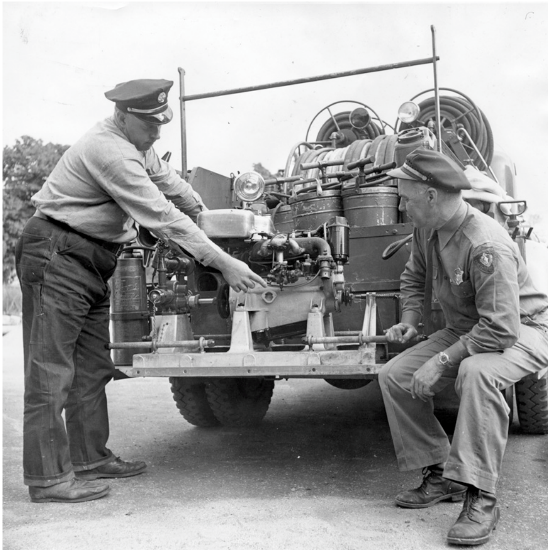
Forest Warden Allan Kidder (left) and District State Warden Arthur Halenborg inspect a new portable pump mounted on the rear of the 1941 Chevrolet Forest Fire Service Truck (Chelmsford Fire Department Collection)
