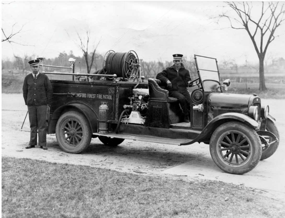
The 1925 Federal Knight double tank chemical car transferred to the Forest Fire Warden's department in 1935 Gil Perham is standing at the rear and Deputy Forest Warden Herb Sturtevant is at the wheel circa 1936 Note the portable pump tucked in the space behind the front seat (Chelmsford Fire Department Collection)
