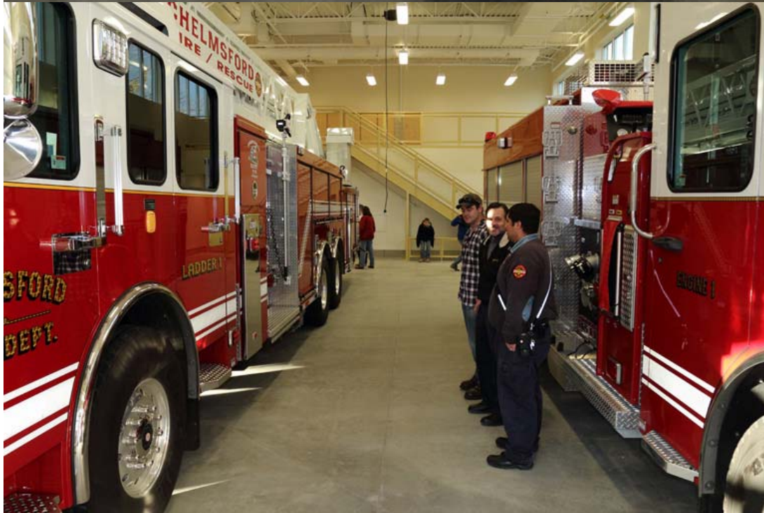
The new Engine 1 is a 2014 Smeal/Spartan Sirius II MFD. The cab & chassis is built by Spartan with the remainder of the body compartments and pump module built by Smeal. The end result is a Smeal class A Pumper with a 1500 gpm pump and a 750 gallon water tank. In addition it carries three ladders: 24' extension, 14' roof, and a 10' for use in attics.
