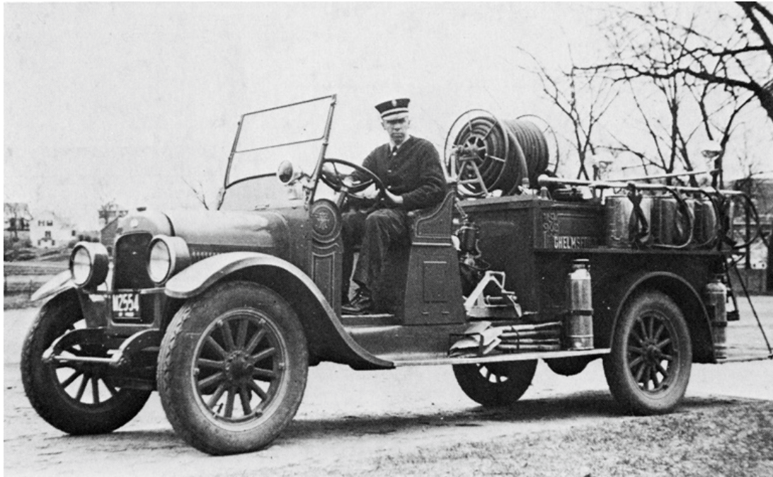
This is the 1925 Federal Knight double tank chemical car purchased for East Chelmsford Gilbert H. Perham is seen here circa 1935 after the truck had been transferred to the Forest Warden's department and modified with a portable pump behind the drivers seat and large hose reel. (Chelmsford Historical Society Collection)
