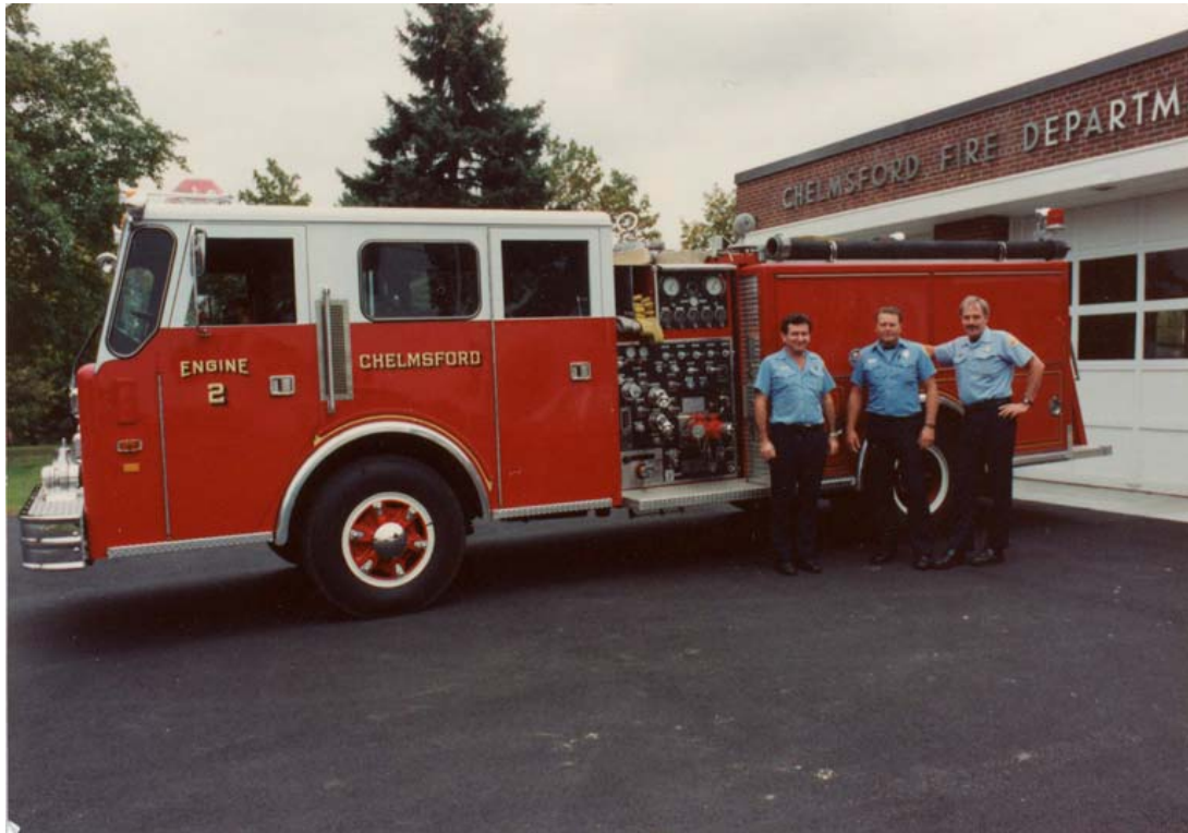
Delivery of this 1976 Mack CF 1,000 g.p.m. Pumper with 500 gal. tank to the Center as Engine 1 started this rotation: (This photo shows the pumper after modifications in 1988 that added a four-door forward cab) The previous Engine 1, a 1972 Maxim 1000 g.p.m. Pumper, was re-designated as Engine 2 and transferred to North The previous Engine 2, a 1966 Maxim 1000 g.p.m. Pumper, was re-designated as Engine 4 and transferred to East The previous Engine 4, a 1951 Maxim 750 g.p.m. Pumper, was placed in Reserve and remained in East Chelmsford (Chelmsford Fire Department Collection)
