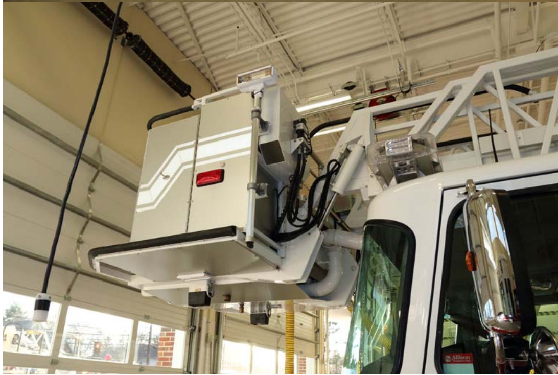
The Ladder 1 truck is a 2013 Smeal/Spartan Sirius Custom EMFD flat roof cab. The cab & chassis were built by Spartan and the remainder of the body compartments and ladder built by Smeal. The end result is a Smeal Ladder truck, sometimes referred to as a Tower. This truck has a 100' steel ladder with a platform at the end. It has a 2000 gpm waterous pump and a 300 gallon tank.
