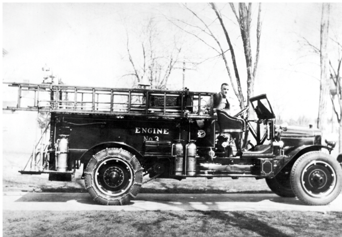
Engine 2, a 1921 Brockway 250 g.p.m. Pumper, was fitted with pneumatic tires and re-designated as Engine 3 at West as seen above, when a new Maxim 500 g.p.m. Pumper was purchased as Engine 2 for North Chelmsford in 1931 Note the chain drive in front of the rear wheel (Chelmsford Fire Department Collection)
